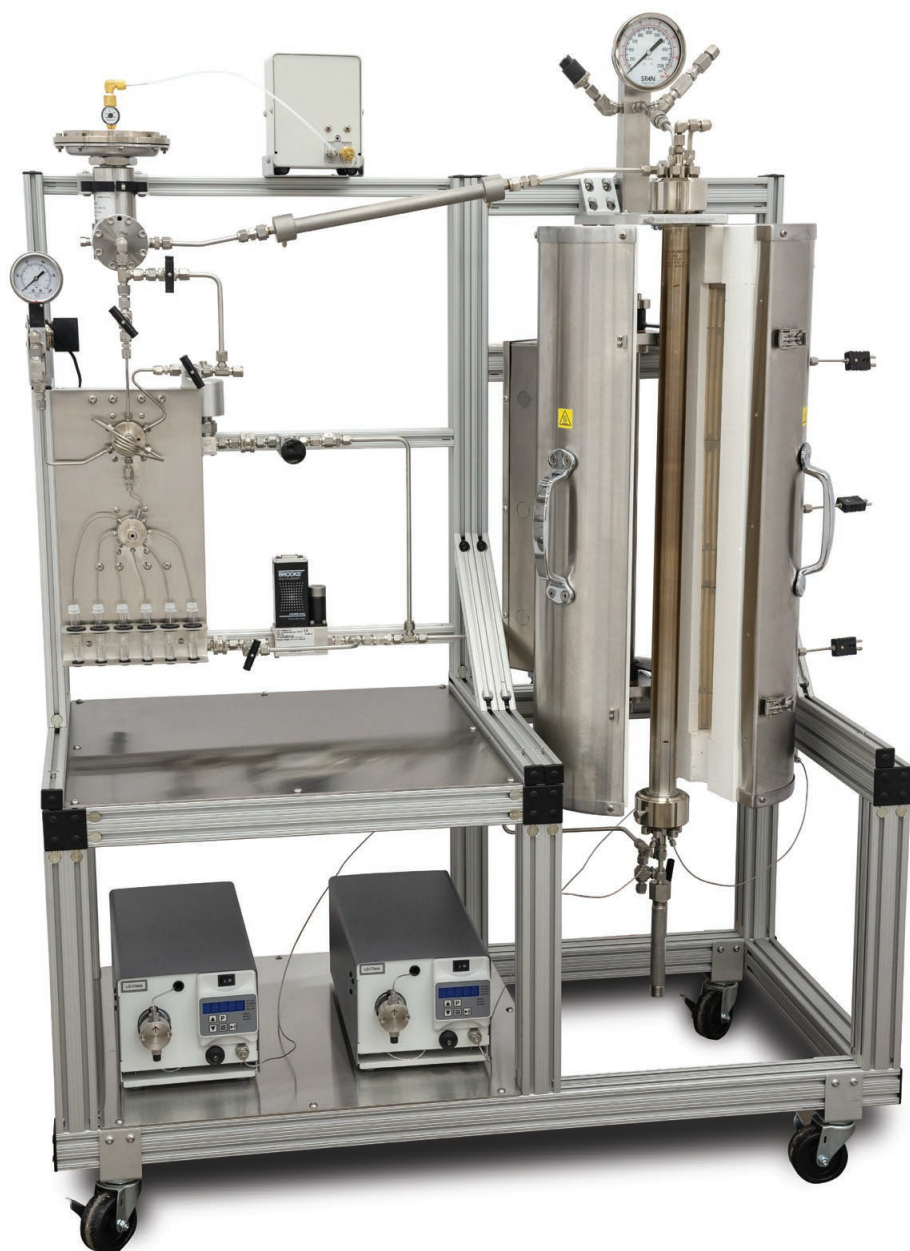
Up-flow 5403 Tubular Reactor System with 300 mL heated volume, one purge line, one gas feed, two liquid feeds, product cooling condenser, and automated 2-phase back pressure regulator. An automated liquid sampler captures representative samples at a user-programmable interval.
