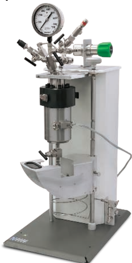
The 500 mL batch supercritical water extraction vessel pictured above is constructed of Hastelloy C-276 and is designed for use to 6000 psi (410 bar) at 400 °C.
