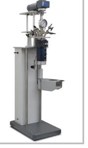
The 4578 Pressure Reaction System shown above and left is a 1.8 L, fixed head reactor mounted on a floor stand and rated for temperatures up to 500 °C with a maximum pressure of 5000 psig. This system is designed to operate in either a vertical or horizontal position.
