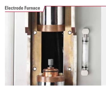
A graphite crucible will be pressed between two electrodes and heated up, in the furnace by using max. 1000 A power. The temperature of the furnace is PC controlled and might reach up to a maximum of 3000  $^{\circ}$ C.
